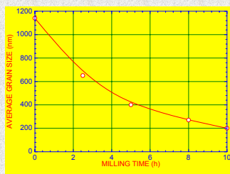
Fig. 2. Average grain size of iron doped TiO_2 as a function of the milling time.
