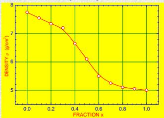
Fig. 2. The density vs. composition of  $x\text{COF}(1-x)\text{PZT}$
