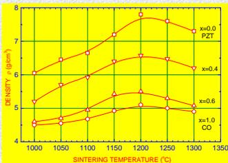
Fig. 1. The density vs. sintering temperature for different composite samples
